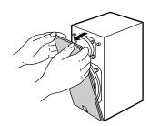
The front cover is fastened to the enclosure at four points and can be removed if desired. To remove the cover, hold on to both sides and slowly pull straight away from the speaker. To reattach, line up the four holes on the inner surface of the cover with the four corresponding pegs on the speaker and push gently.
