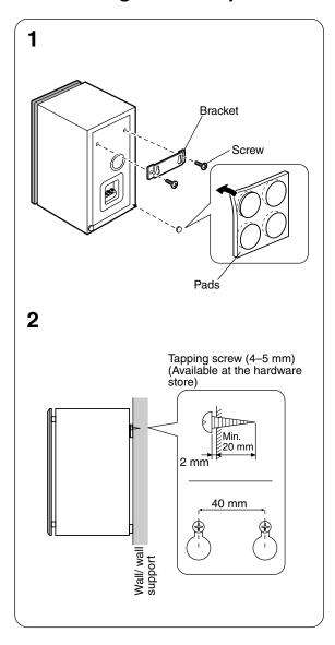
Mount the rear speakers on a shelf, rack or directly on the floor, or hang them on the wall.
