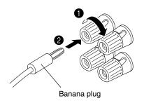
For connections, keep the speaker cords as short as possible. Do not bundle or roll up the excess part of the cords. If the connections are faulty, no sound will be heard from the speakers. Make sure that the + and – polarity markings of the speaker cords are observed and set correctly. If these cords are reversed, the sound will be unnatural and lack bass.
